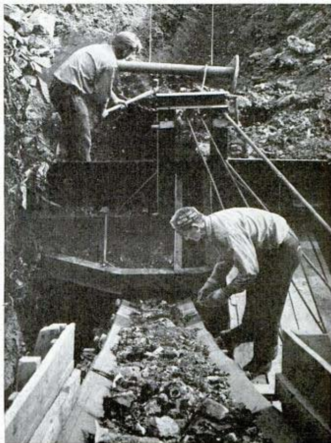
Below, operators watch the material as it is drawn from the junk pile by the main conveyor
